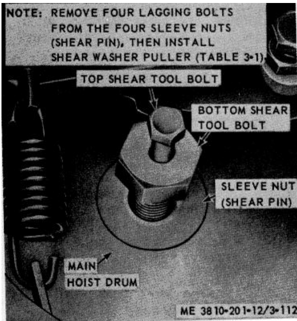
Figure 3-112. Sleeve nut, removal and installation.
